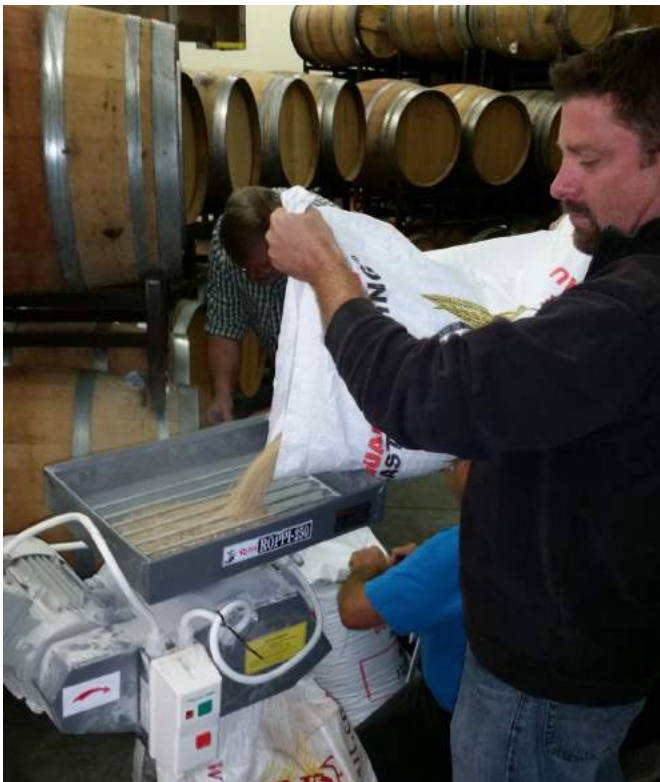
This hanger queen Hungarian grain mill has a big motor, maybe 2hp, running on 240v. Lotsa torque there!
