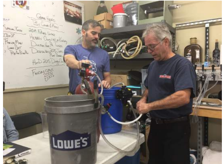
Craig's pump for liquid transfer requires no electricity, doesn't need to be primed, and is much cheaper than the most brewing pumps!
