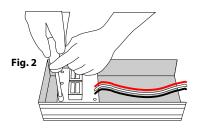
**4.** Lift the old power supply off the circuit board and discard.
