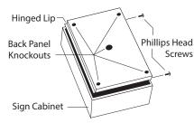
2. Place the back panel on the wall surface using a level to make sure it's straight. Use a pencil to mark the locations of the mounting holes on your wall surface. Drill your wall surface. The diameter of the (4) four corner mounting knockouts is 1/4" and the conduit knockout is 7/8".
