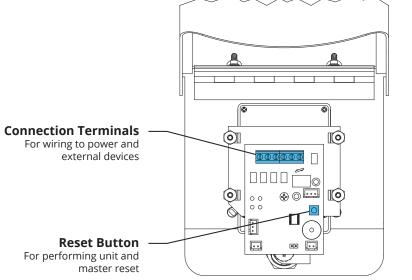
Unit shown with front panel fully open. Internal wiring not shown for clarity.
