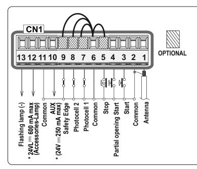
WARNING: The control unit is designed for the automatic detection of not used N.C. inputs (Photocells, Stop and Limit switch) except for the SAFETY EDGE input. The excluded inputs during the self-programming can be restored through the «INPUT STATUS CHECK» menu (chapter 15) without need to repeat the control unit programming
