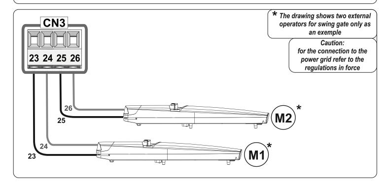
Fuse 3,6A delayed on 230V~ power supply Fuse 6,3A delayed on 115V~ power supply
