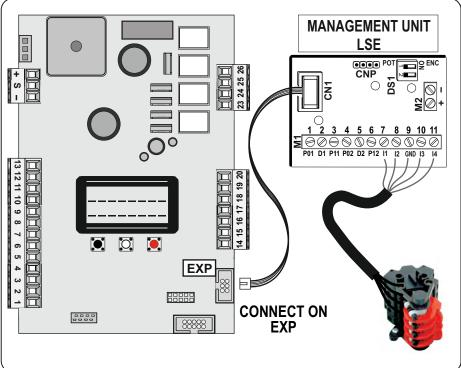
The **«LSE»** management unit can be connected through the **EXP** connector
