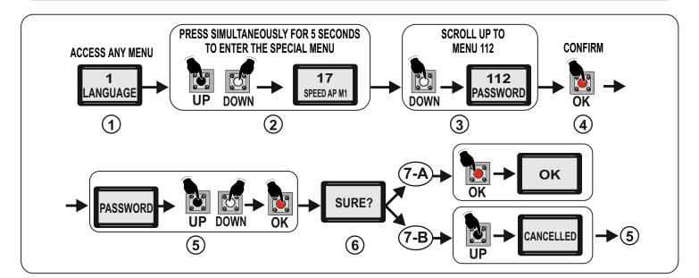
Once the password is activated, **the menus will only be shown but cannot be adjusted**; To unlock the control unit enter the correct password in the 112-PASSWORD Special Menu.
