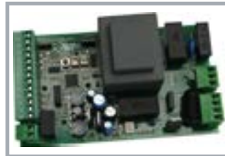
Analogue control unit with programming through dipswitches and Trimmers
