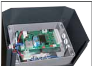
Electronic control unit positioned on the top of the carter
