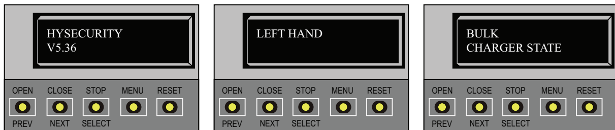
Example of Operator Status Displays
