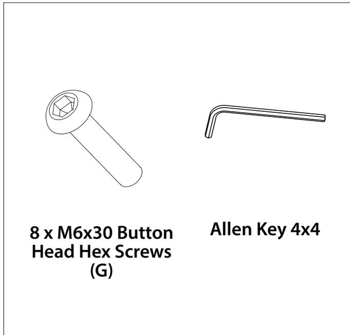
**4** Connect the left and right columns to the feet. Tighten the screws(G) with a 4x4 allen key.
