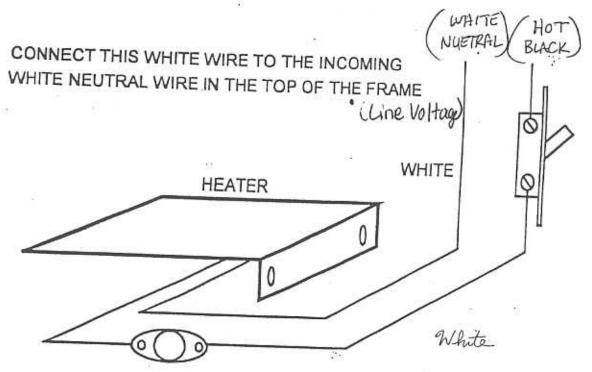
CONNECT THIS WHITE WIRE TO BOTTOM SCREW OF ON / OFF SWITCH
