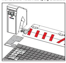
Anchoring the WedgeSmart DC
