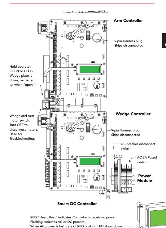
Connect DC Wire Harnesses on both Controllers.
