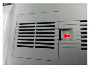
2. Remove the air filter, wash it with warm water thoroughly, dry it completely, and replace. If the filter begins to deteriorate during washing, it is advised you purchase a new one from an Authorized IDP Dealer.
