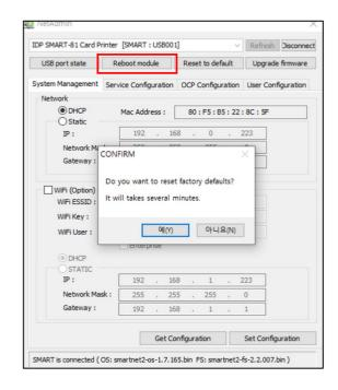
Figure 69 Rebooting network module
