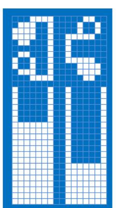
The left side shows the remaining balance of the re-transfer film, and the right side shows the remaining balance of the ink ribbon. If an 'X' is displayed, it designates that no ribbon was found, or it was installed incorrectly.
