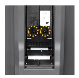
Figure 21 Adjusting card thickness lever
