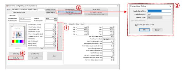
Figure 94 Printer head setup
