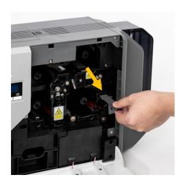
Figure 11 Take out cleaning roller Cartridge
