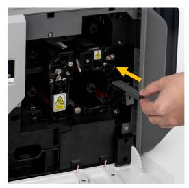
Figure 15 Installing the cleaning roller cartridge
