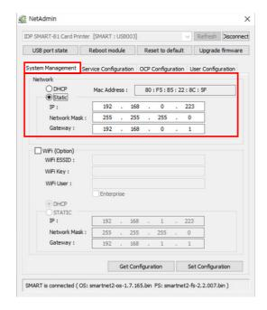
Figure 74 DHCP / Static IP configuration
