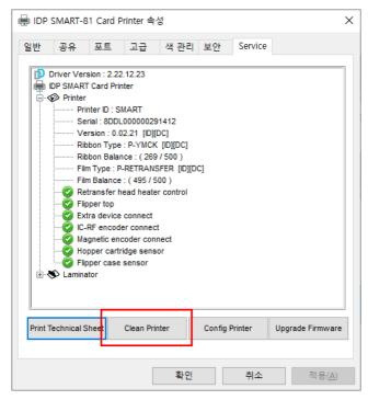
**Step 1**: Connect the SMART printer to a PC, turn it on, and prepare the cleaning card. Click "Start cleaning" to move on to step 2.
