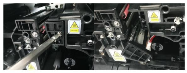
Figure 95 Printer head disassemble
