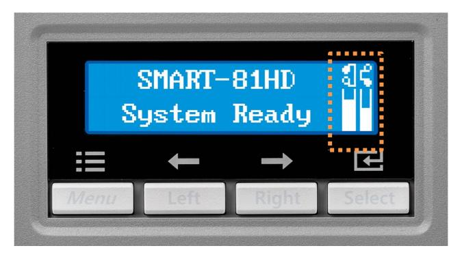
Figure 6 SMART-81 Display and Buttons
