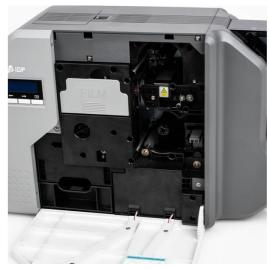
Figure 16 Installing film cartridge
