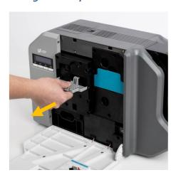
Figure 9 Remove film cartridge
