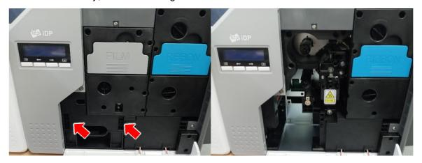
Figure 39 Remove module (IC, RF)
