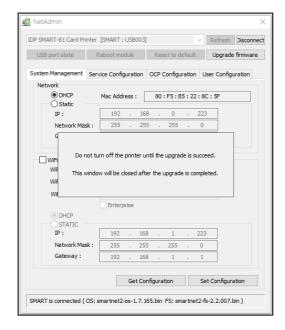
Figure 72 Upgrading the firmware 2
