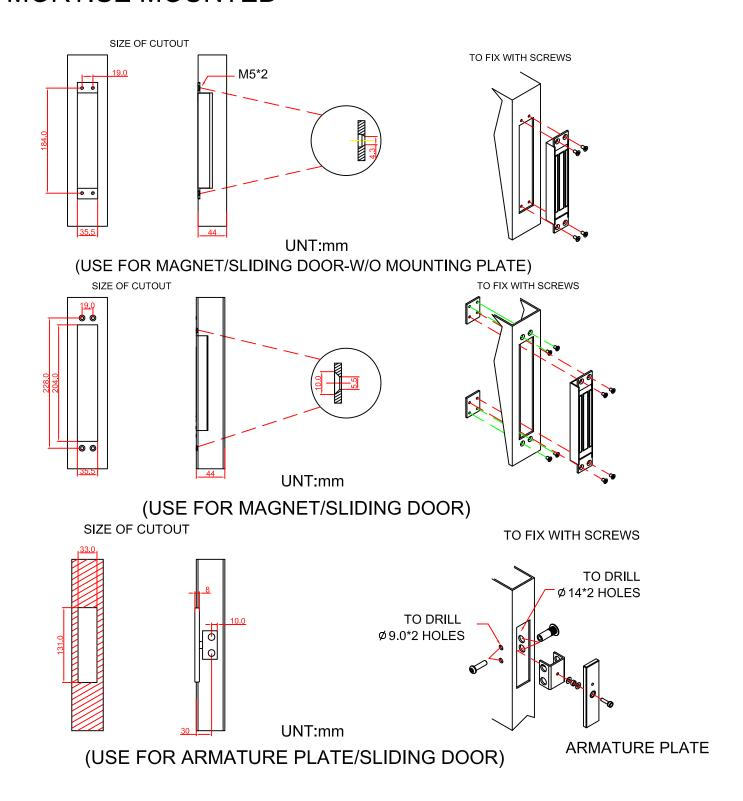
★★Important: Fix the armature plate not too tightly,and make the rubber washer more flexible,in order to make the armature plate automatically adjust its proper position with the magnet.
