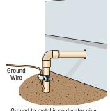
**IMPORTANT:** Ground wire shown without safety protection for clarity. Make sure ground wire is protected from being touched or electrical shock could occur!
