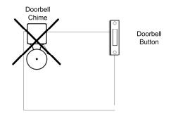
**Step 2:** Go to the existing doorbell and disconnect the wires. Splice the 2 wires together.
