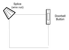
**Step 3:** Remove the existing doorbell button. Replace it with the Door box using the same 2 wires. Note which wire you connect to (+) and (-).
