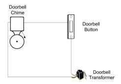
**Step 1:** Locate the doorbell's transformer. Disconnect the low voltage wires from the transformer.
