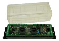
The DP38-CI DoorBell Fon **Inbound Relay Trigger Controller** module will give you 0.6 to 3 seconds dry-closure when the Door Station button is pushed. This add-on module will allow your doorbell or any other external trigger devices to be activated along side your phone.
