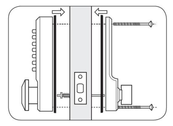
• The spring loaded spindle will fit doors between 55mm (2 3/16") and 70mm (2 3/4") thick. For doors less than 55mm (2 3/16") remove the 15mm (9/16") break-off end of the spindle. The spindle will then fit doors between 40mm (1 9/16") and 55mm (2 3/16"). The spring keeps the spindle firmly engaged and prevents it moving out of engagement with either of the plates.
