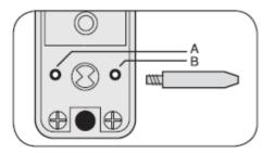
• Fit the deadbolt support post in hole A for a right hand hung door, or B for a left hand hung door. Your door is
