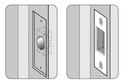
• Position the keeper plate on the frame so that it lines up with the deadbolt.
