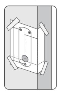
Note: Ensure enough room for the latch support post Please align the template to suit the locks backset: 60mm (2 3/8") standard or 70mm (2 3/4").
