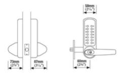
Model CL620/625/650 With full 'Panic Function' mortice lock & cylinder
