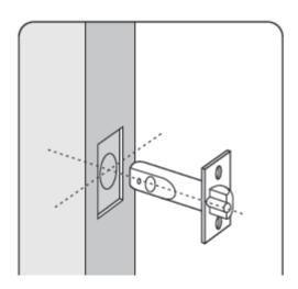
Note: Space required above latch body for cam to rotate.
