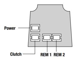
**REM 1** is for connection to a reception desk push button or a door intercom system. Pressing the button will cause the keypad to flash blue on the lock and release the lock for the pre-set time.
