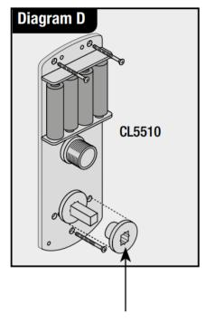
Alignment insert MUST be removed before completing installation.
