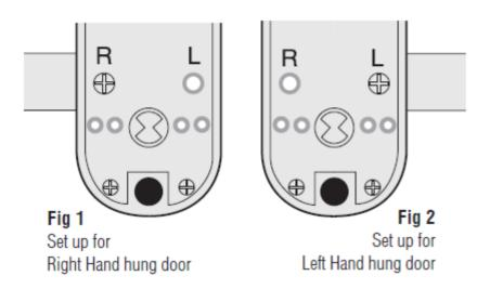
**7.** Fit the CL500/505 front unit with the two fixing bolts. Insert the spindle with the flat blade into the CL500/505 front unit, ensuring that the blade is at the correct angle for the hand of door: see diagram.
