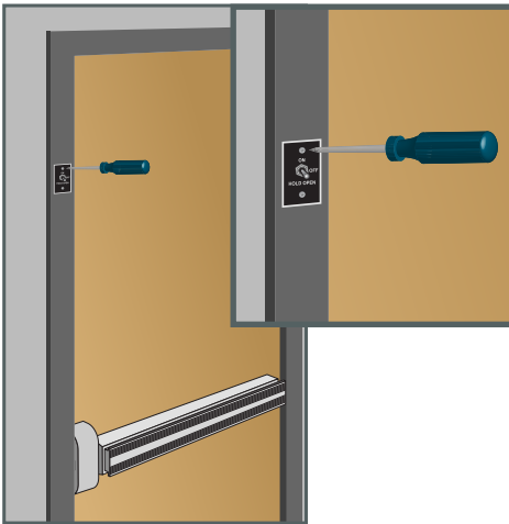
ON / OFF / HOLD OPEN Switch installed
