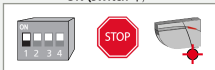
RELAY 1: STOP-impulse on swing side of door
