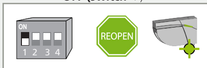
RELAY 2: REOPENING-impulse on approach side of door
