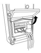
**1** Slide down and then open the cover, and connect wires to the terminal block.
