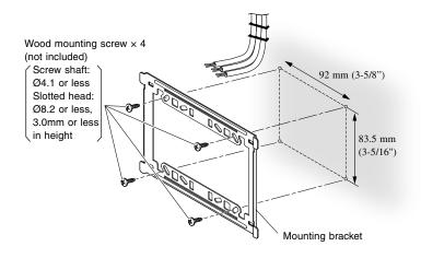
\* To pass the wire through the back of the station, cut out the cable inlet.
