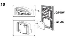
**10** For the GT-SW and GT-AD, remove the resident name/address plate or paper by pressing either the left or right end. (Peel off the plastic film.)Use a permanent pen to write the resident name and address on the transparent plate and mount the plate on the module.
