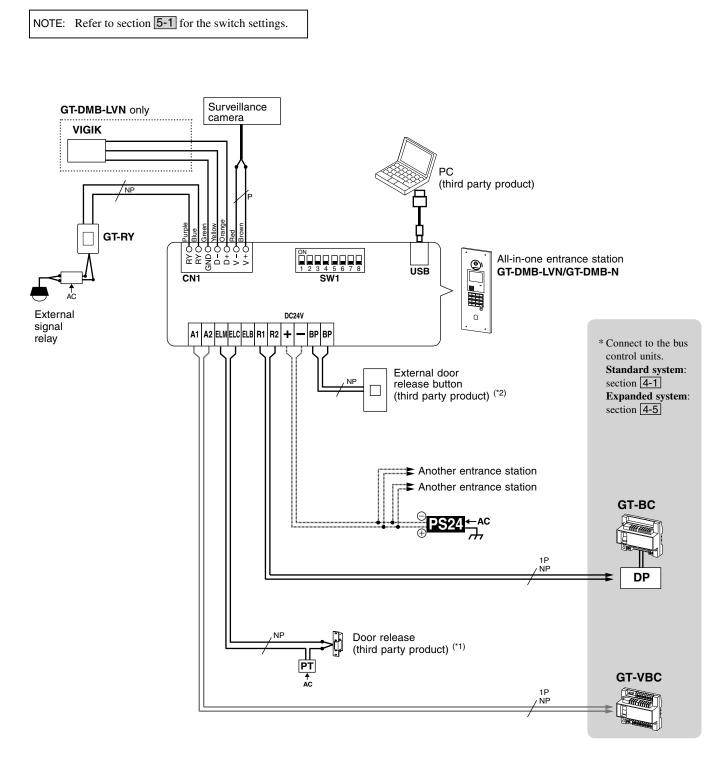
(\*1): N/C (Normally Closed) [ELB, ELC] N/O (Normally Open) [ELM, ELC] Less than AC/DC 24V, 4A (resistive load)
