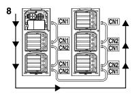
**8** Attach the connection cables between the modules. Mount modules on the back boxes.
