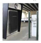
**Features** The reader's 2-color LED and beeper are controlled by the reader itself. No external wiring is required for this feedback.
