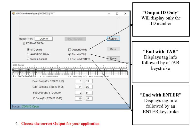
Whether you are enrolling tags into your access control system, or creating a database of current users, you can modify the program to adjust the output that works best for you.
