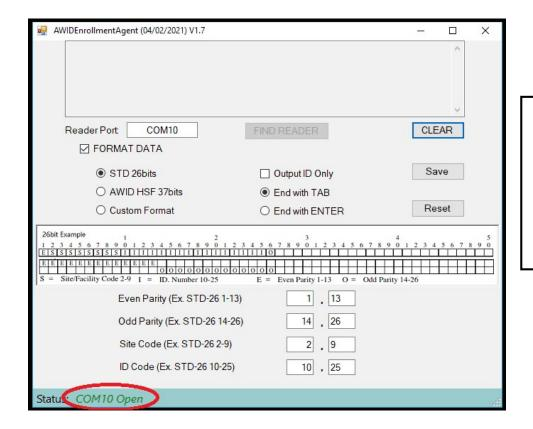
Once the reader is connected, the status bar will illuminate green and display "COM Open"
