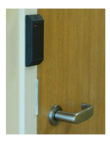
Features The SR-2400 reader contains a 3-color LED and a 4 kilohertz beeper. Both LED and beeper are controlled by the reader itself, and also can be controlled externally by the host system. The LED can indicate access-granted by the host. The beeper can be used as an alarm that prevents further card reads until the alarm condition is cleared.
