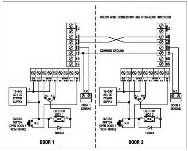
An inter-lock system needs two door controllers. This application example uses two Post Mount Keypad with simple cross wire connection on the "Output 1 Inhibit" and "Inter-lock Control Output" terminals. It is necessary to link up the "(-) GND" terminals of the two keypads as common ground to achieve the inter-lock logic function.
