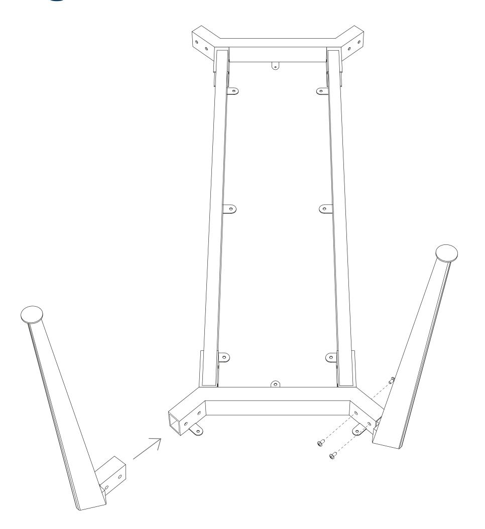
**Tip:** Your legs should sprout outwards, like the diagram above
