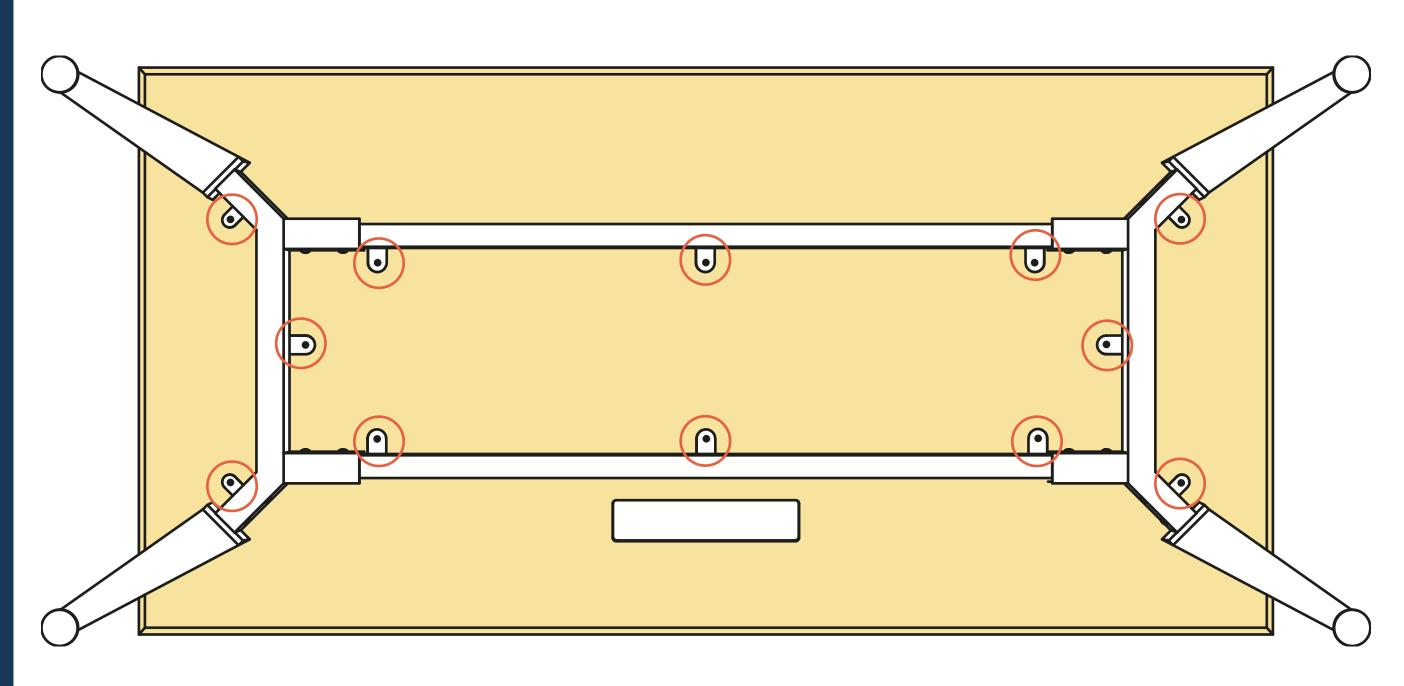
**TIP:** Use the pre-drilled holes on the corners of the desk to center and secure your desk to the base. The center screws are optional, and can be screwed directly into the table top.
