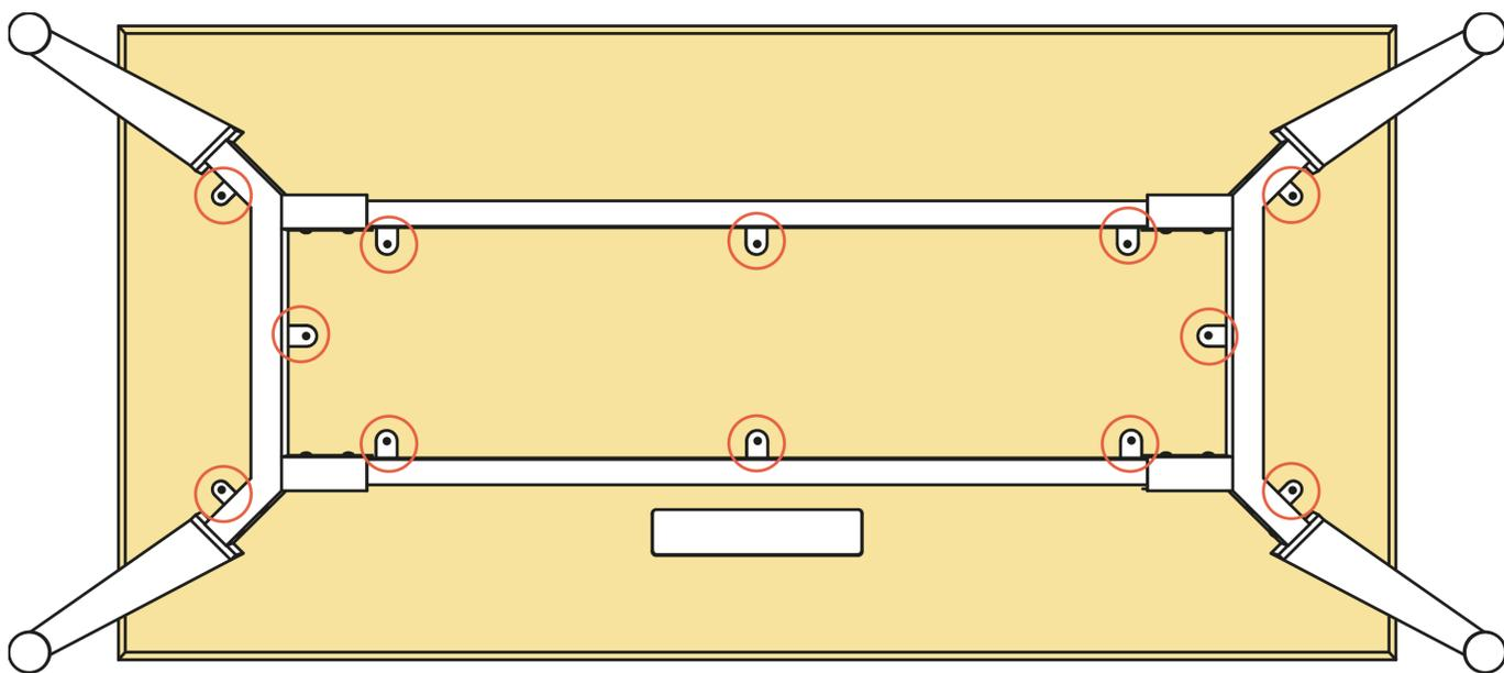
**TIP:** Use the pre-drilled holes on the corners of the desk to center and secure your desk to the base. The center screws are optional, and can be screwed directly into the table top.
