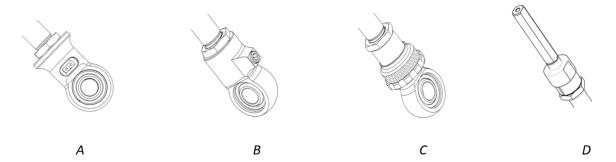
**Eyelet Adjuster** – There are several options for the eyelet adjuster as displayed above. This adjusted can be used for a 1-way rebound, compression and a combined rebound compression adjuster. This eyelet adjuster is used for rebound as stander across most shock models. It will be specified to you if this eyelet adjuster changes other damping characterises
