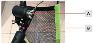
Adjust this nut to set the correct friction on the ball arm.
