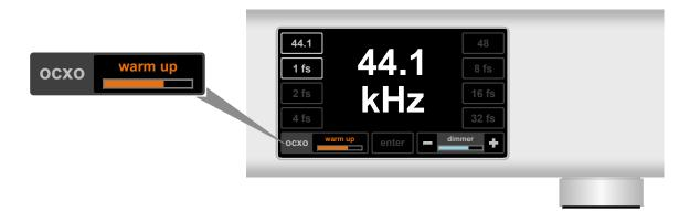
The warm up time of the **NADAC C** will vary depending on the ambient temperature. Typically, the warm up time is approximately three hours at an ambient temperature of 25 C°.
