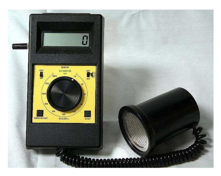
Geiger detector probe sensitive to alpha and gamma radiation, and with high sensitivity to Beta particles.
