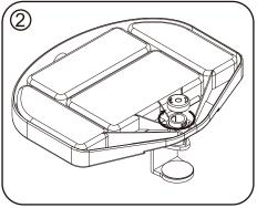
Lock the cap on the bottom of the C-clamp
