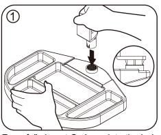
Forcefully insert C-clamp into the hole on the tray as shown in the picture
