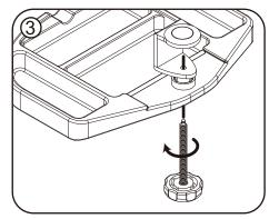
Insert screw into the C-clamp
