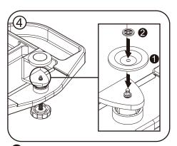
Forcefully insert C-clamp into the hole
