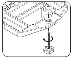
Insert screw into the C-clamp
