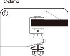
Tighten the screw to secure the tray onto a desk
