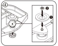
Place the metal plate on the screw
