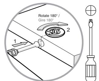
Turn minifix cams to the right to tighten.
