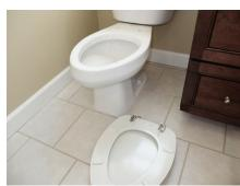
Remove the 2 bolts that attach the existing toilet seat to the toilet basin. Remove the toilet seat and set it aside. Clean the top of the toilet basin with an anti-bacterial cleaner.
