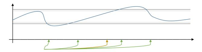
The blue curve corresponds to the measured analog signal. The orange curves correspond to the analog measurements. The green curves represent the sending of the measured analog value which has just crossed a threshold. The yellow curve represents the sending of the measured analog value when the 'temperature feels' is reached.
