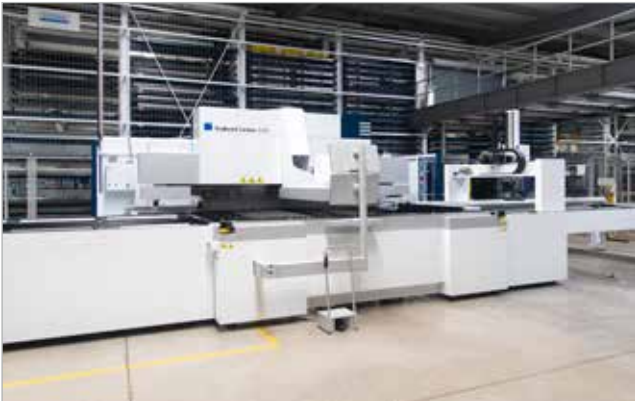
Automated bending center TRUMPF
