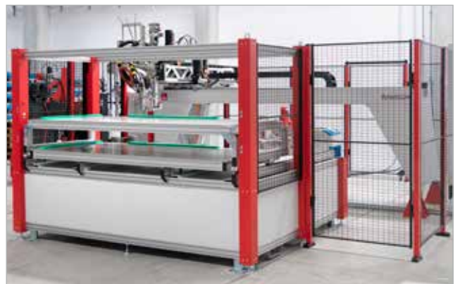
Center for glass gluing and cabinet door seal applications for switchboards
