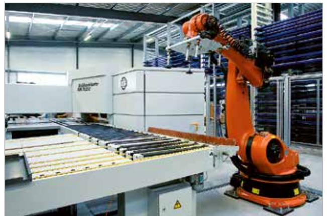
Automated bending center RAS
