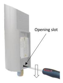
The housing must be opened to access both the terminal block and the mini-USB port used to configure the module.
