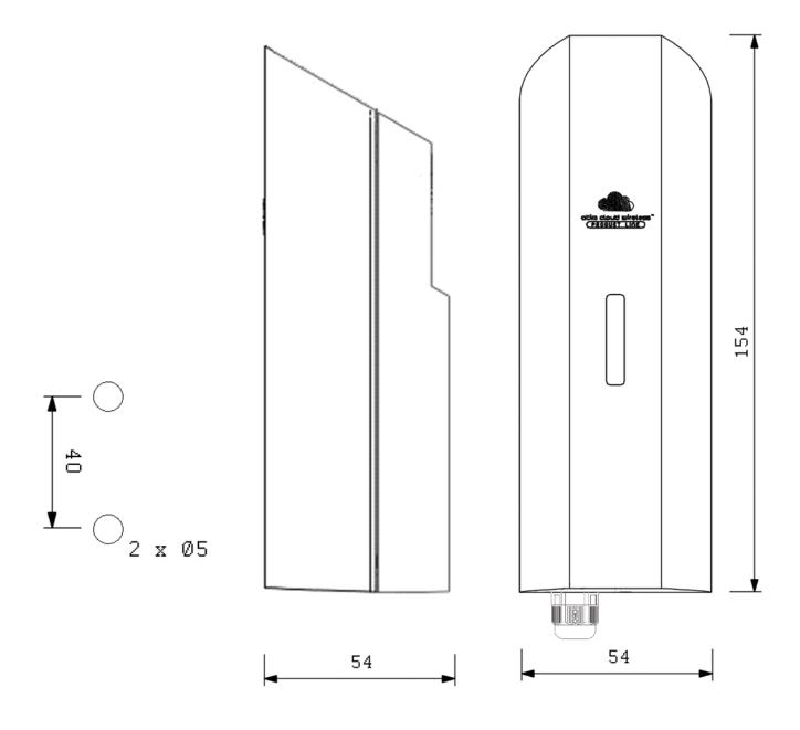
Maximum cable diameter through cable gland: 7 mm
