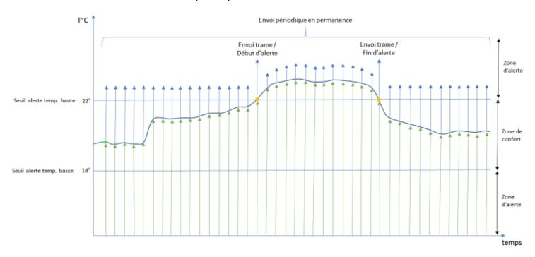
On the other hand, because this mode involves regular (and potentially very frequent) radio transmissions, this mode of operation may consume large amounts of energy, leading to reduced battery life.
