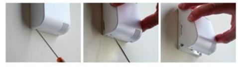
\* It is imperative to open the case from below; opening from the top can damage the circuit.
