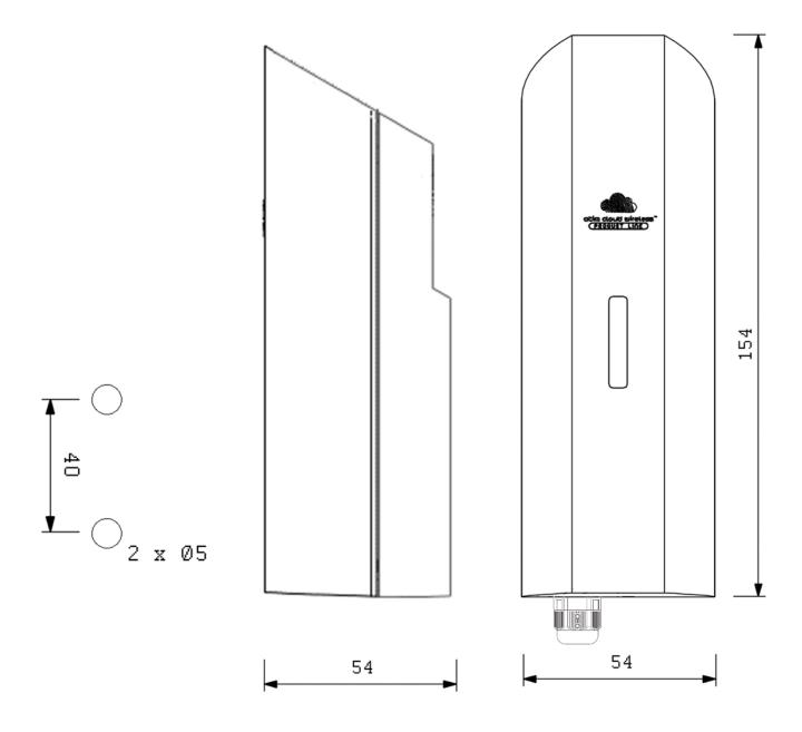
Maximum diameter of the cable in the stuffing box: 7 mm.
