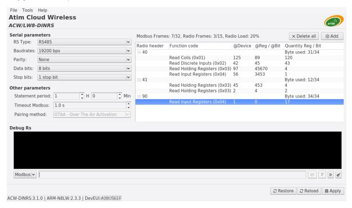
In this example, we have 3 radio frames with headers of 40, 41 and 90 plus 7 Modbus frames. Radio frame 40 contains 4 Modbus frames; radio frame 41 contains 2 Modbus frames; and radio frame 90 contains just one Modbus frame.
