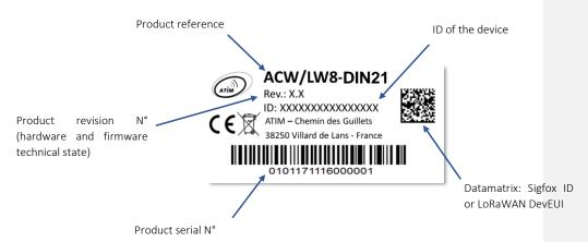
Each product in the ATIM ACW range has a QR Code label visible either on the side or on the front of the product. This QR Code can be easily read with any 2D barcode reader application on a smartphone.
