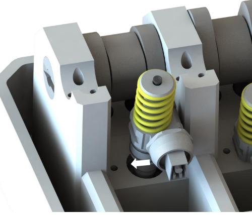
Note: The professional revision and disassembly of the unit injectors requires the use of new screws and sealing elements. If required, selected complete sets of consumables in excellent quality are available at the following link:
