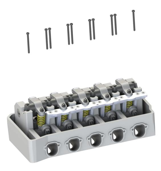
step 21: insert rocker arm expansion screws – new screws have to be used!
