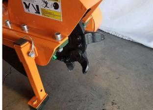
Grinding wheel. Used for grinding the stump.
