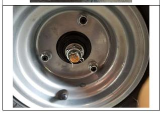
Install washer, nut, and cotter/lock pin.
