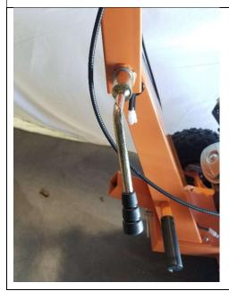
Clamp for adjustable bow handle. Used to loosen the bow handle, make adjustment to bow handle, and tighten to keep secure.
