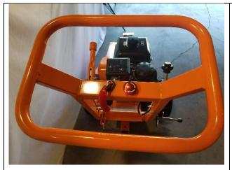
Adjustable control handle with emergency palm stop switch and emergency pull switch.
