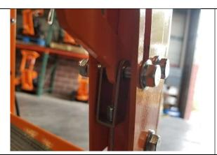
Install bolt, washer, and nut into brake cable/brake arm.
