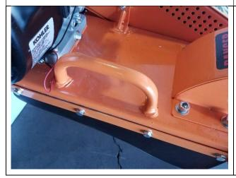
Lift handles. Used to assist when carrying the unit into a trailer.
