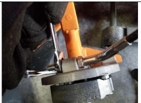
Tighten adjuster and lock nut.
