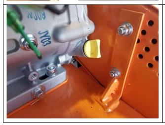
Oil reservoir dip stick. There is one on each side of the engine and they both go into the same reservoir. This is used to fill the engine with oil. Can also be used to check and make sure the correct amount of oil is used. The bolt on the bottom left of the photo is used to drain the oil. Use aluminum foil to direct the oil to a container to keep the unit clean.
