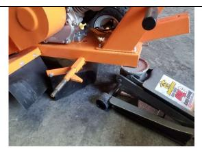
Place a floor jack under left rear corner of stump grinder. Lift enough to install tire.
