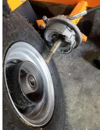
Install wheel with brake drum.
