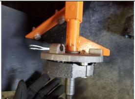
Slide brake pad assembly on to the axle and line up notch to keep from spinning. Brake pad assembly can be found in the green accessory bag.
