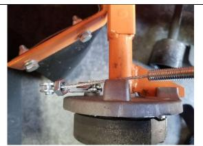
Loosen lock nut and install brake wire and brake adjuster into brake adjuster mount.
