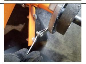
Install brake cable end into holder.
