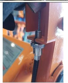
Adjust barrel adjuster to be able to slide in the brake cable.
