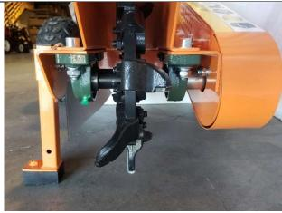
Pillar bearing. These bearings let the grinding wheel spin. Grease the bearings about once per season using bearing grease.
