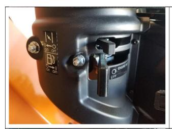
Top lever is Choke and bottom lever is Fuel. Choke is used to close the air way and enrich the fuel mixture ratio. This is used during cold starts to assist the engine during start up. The Fuel lever is to allow fuel from the gas tank to the carb. It is also used to shut off the machine.
