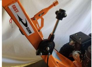
Locking throttle adjustment. Used to raise and lower engine and grinding wheel speed.
