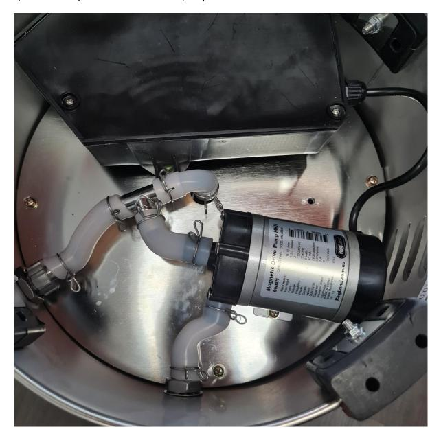
Make sure there are no kinks or twists in the silicone hosing which could impede the flow of liquid. If a kink is present then this may result in a pressure build up and the hose eventually splitting.
