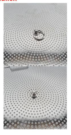
TIP: For easy removal of the false bottom from the boiler press down on one side of the false bottom while lifting from the eye bolt assembly
