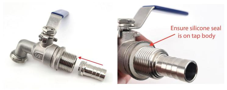
Then turn the BrewZilla upside down and insert the thread of the tap through the pre-drilled hole in the boiler. Secure the tap on the inside of the boiler using the hex nut and secure the barb in place by tightening the retaining nut onto the taps thread.
