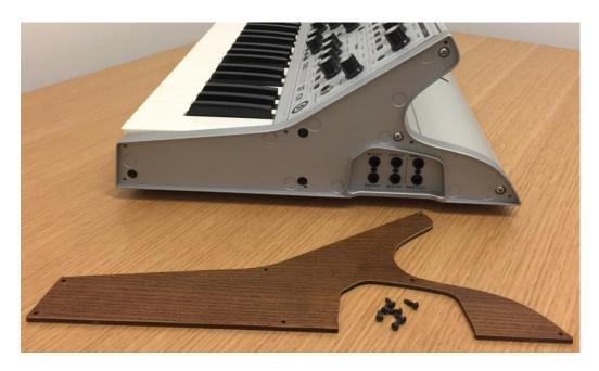
Referring to step 5 above, insert the blunt machine screws through the end panels and slip the felt washers over the screw tip. Next, slip the white spacer over the tip of each screw so that the spacer rests against the face of the felt washer. Continue with assembly as normal.
