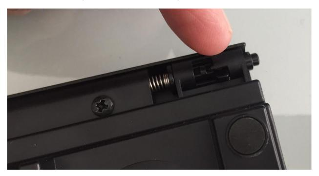
Insert the synth into the upper cradle, ensuring that the pin pops into the hole.
