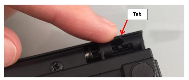
Push the tab towards the middle of the synth (to the left in this photo). With the tab moved to the left, rotate it away from the front edge (down in this photo).
